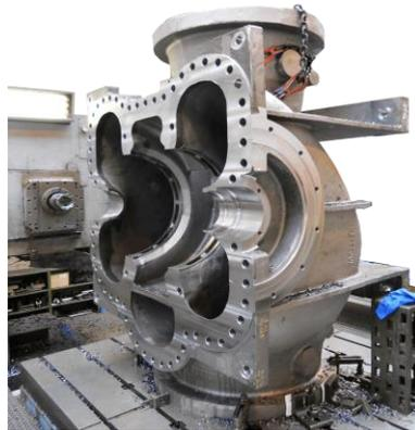
After machining, Casings are then assembled and line-bored, if required then static pressure tested.
