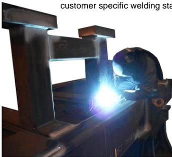
Weld sequencing and vibratory / thermal stress relieving is used to reduce stress and minimise distortion in the large fabricated steel structures. Non-Destructive Testing is conducted to suit customer requirements.
